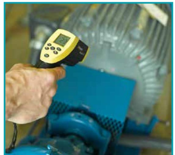
IPS field service technicians use state-of-the-art technologies and test equipment for the most accurate predictive maintenance results. On-site diagnostics include vibration analysis (left) and laser temperature readings (right).
