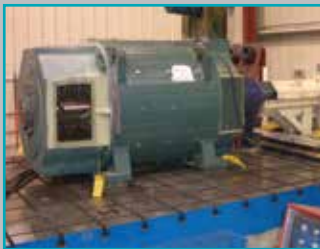
Load testing to 1,750 HP and 7,200 VAC / 750 VDC
