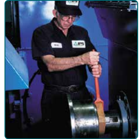
We rotate shafts on a monthly basis (or to customer specification)
