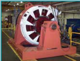
Run testing to 7,200 VAC / 700 VDC
