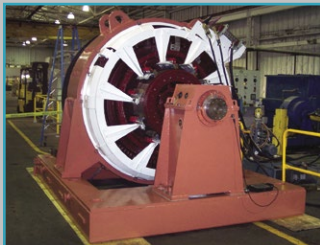
Run testing to 7,200 VAC / 700 VDC
