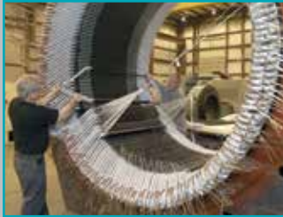
IntegraCoil™ 15 kV stator rewind
