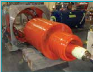
DC motor rewind
