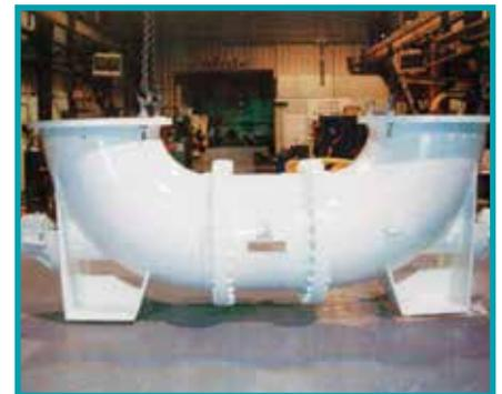
*Remanufacture of 38" Pump with 316 stainless steel inside liner for an 800 HP / 450 RPM circulating pump*
