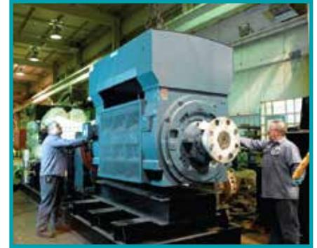
*New 2,500 HP / 4,160 V induction motor installed on diesel generator skid – total skid weight: 37,500 lbs.*
