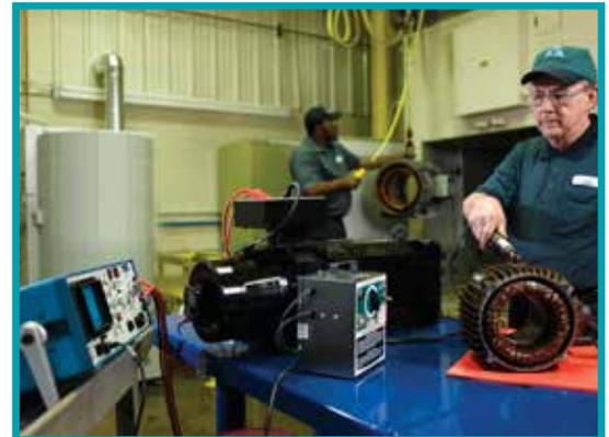
*Self-contained small motor repair departments include parts washers, ovens, balancing and testing equipment*
