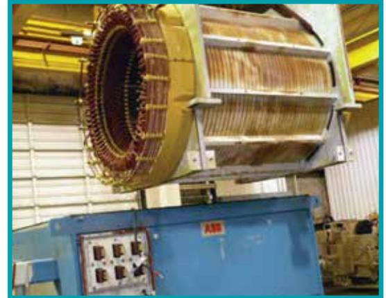
*18,500 HP, 13.8 kV stator being removed from enclosure*
