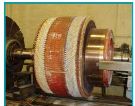
*Rewind and rebuild of a 20,000 lb. / 1,750 HP / 500 VDC mining hoist motor*
