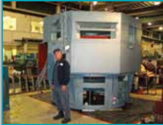
Testing to 750 kVA - 4,160 V, 500 VDC
