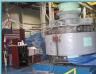
No-load testing to 25,000 HP and 13.8 kV / 750 VDC
