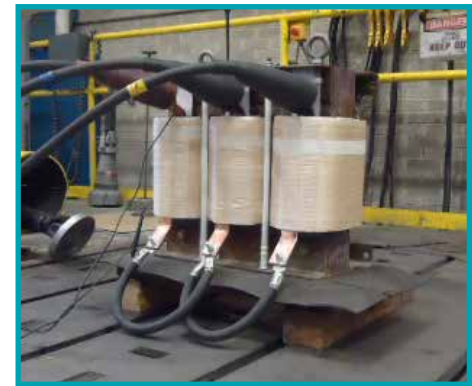
All line reactors are tested before and after remanufacture
