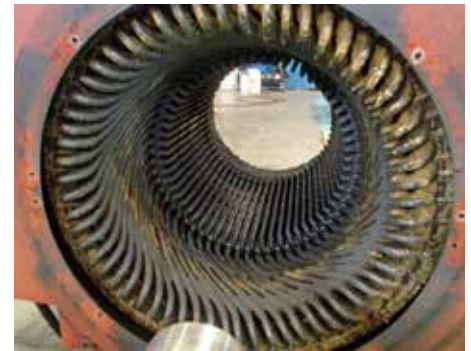
Before: PowerSeal windings received covered in oil & dirt
