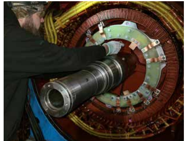
The IPS engineered upgraded rotor connection is designed to accommodate stretching connectors without fatigue.
