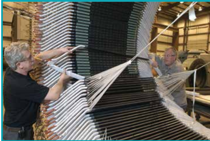
IPS Cleveland provides ABB authorized "global VPI" and "B-stage" rewinds up to 13.8 kV. Our premium "global VPI" rewind technologies, including EnduraSeal, PowerSeal and MegaSeal, are backed by an industry-leading 5-year winding warranty
