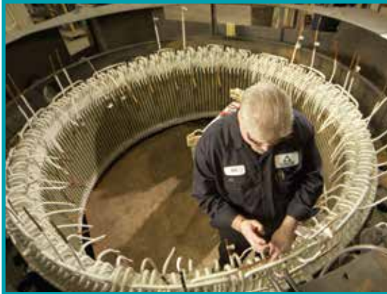
IPS offers exclusive EnduraSeal®, PowerSeal™ and MegaSeal™ "global VPI" rewinds up to 13.8 kV, including an industry leading 5-year stator winding warranty
