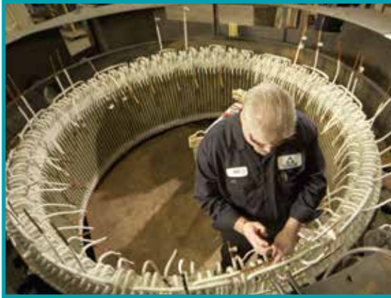
IPS offers exclusive EnduraSeal®, PowerSeal™ and MegaSeal™ "global VPI" rewinds up to 13.8 kV, including an industry leading 5-year stator winding warranty
