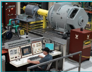
Load testing to 1,500 HP and 7,200 VAC / 700 VDC
