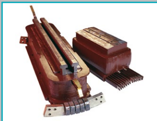
Remanufactured field coils - edge and wire wound
