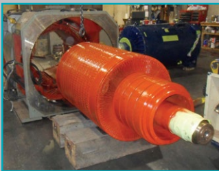
DC motor rewind
