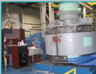
No-load testing to 25,000 HP and 13.8 kV / 750 VDC
