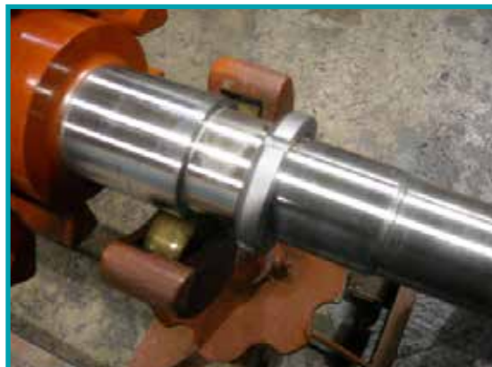
Bent drive shaft resulted in bearing preloading, overheating and failure
