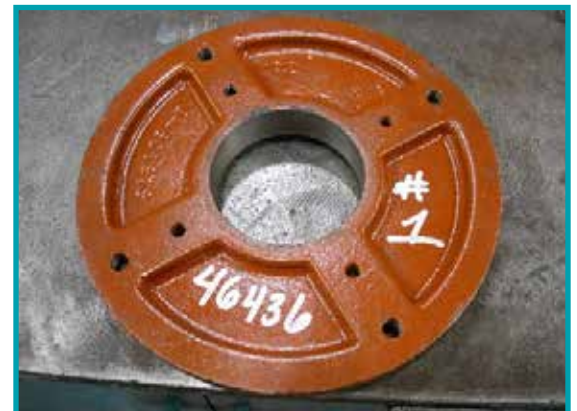
Improperly machined drive end bearing housing caused misalignment
