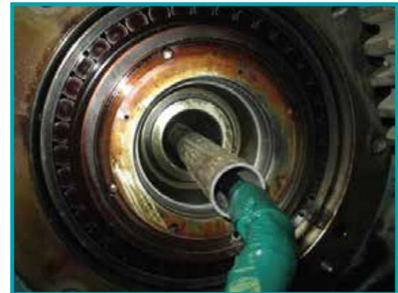
*IPS can replace downwind, low-speed bearings in conjunction with the gearbox seals.*
