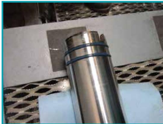
*Faulty seals that cause slip ring issues due to gearbox oil contamination are easily replaced up-tower*
