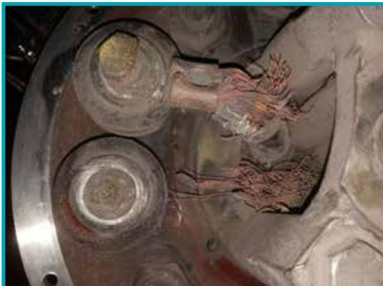
*Failed wind generator rotor leads*
