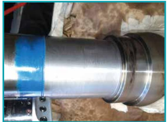
*IPS utilizes steel sleeving instead of typical and less reliable epoxy repair of journals and shafts*
