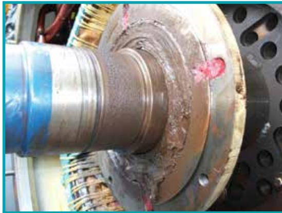
*Bearing spinning on the shaft? Why not repair up-tower using our proven and reliable shaft repair service?*
